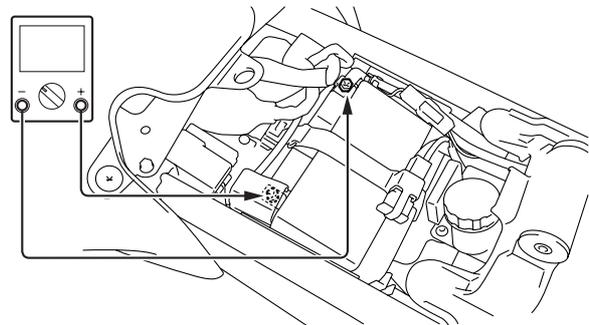
5. Connect the test coupler adapter "1" to the ABS test coupler "2".
