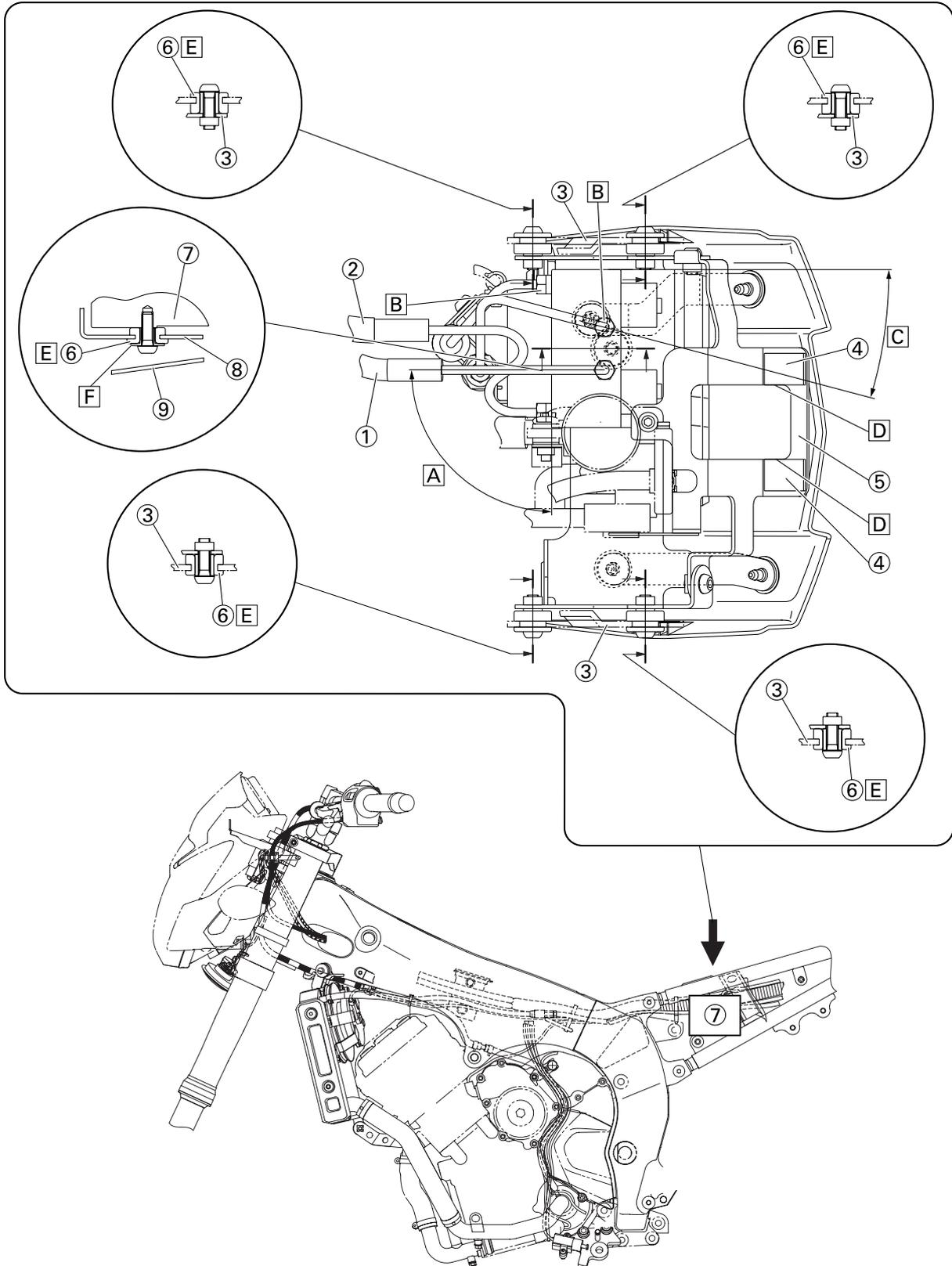
1. Brake pipe/joint assembly (front brake master cylinder to hydraulic unit)
