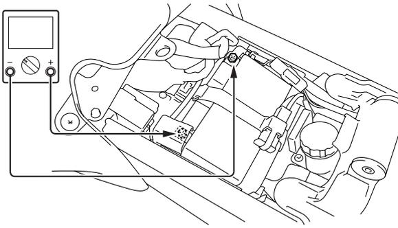
5. Connect the test coupler adapter "1" to the ABS test coupler "2".
