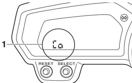
4. After selecting “CO”, simultaneously press the “SELECT” and “RESET” buttons for 2 seconds or more to execute the selection.
