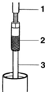
11. After filling the front fork leg, slowly stroke the damper rod "1" up and down (at least ten times) to distribute the fork oil.
