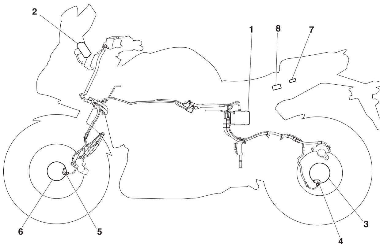
1. Hydraulic unit assembly (ABS ECU)
