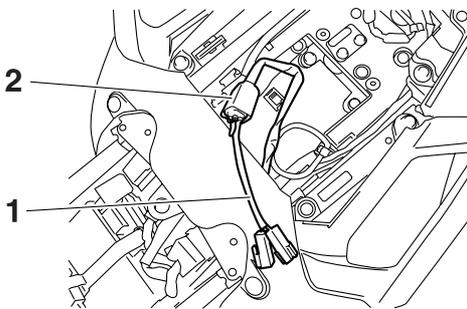
6. Set the engine stop switch "1" to "⊗".
