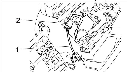
2. Turn the main switch to "ON". Fault codes will be displayed in the multi-function display.
