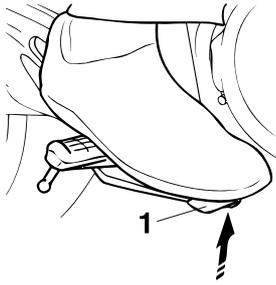
12. After the pulsating action has stopped in the rear brake pedal, it is generated in the front brake lever 0.5 second later and continues for approximately 1.5 seconds.
