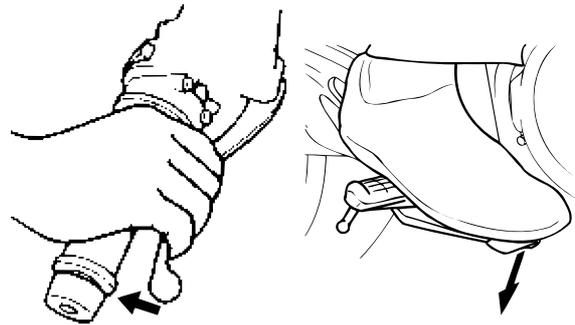
10. A reaction-force pulsating action is generated in the front brake lever "1" 0.5 second after the brake lever and brake pedal are operated simultaneously and continues for approximately 1.5 seconds.
