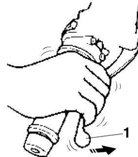
11. After the pulsating action has stopped in the front brake lever, it is generated in the rear brake pedal "1" 0.5 second later and continues for approximately 2 seconds.
