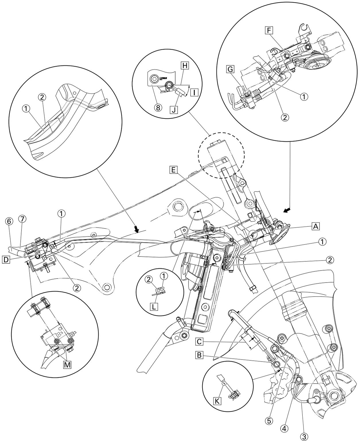
1. Brake hose (hydraulic unit to front brake calipers)
