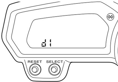
3. Press the “SELECT” button to select the CO adjustment mode “Co “1”” or the diagnostic mode “dl”.
