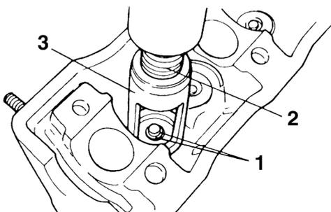
5. To secure the valve cotters onto the valve stem, lightly tap the valve tip with a soft-face hammer.
