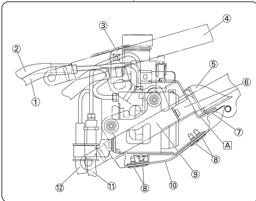
1. Brake pipe/joint assembly (front brake master cylinder to hydraulic unit)
