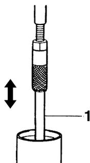
12. Before measuring the fork oil level, wait ten minutes until the oil has settled and the air bubbles have dispersed.
